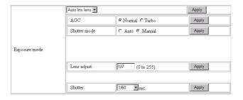
**CCD Iris:** Select this option when you use a fixed-iris lens to adjust the exposure using the electronic shutter and AGC (Automatic Gain Control).
